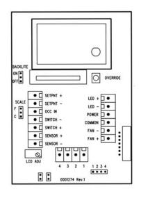
The Continental Series can be customized to work with any building automation system. Because of this there are many possible connection configurations. The above represents the standard configuration. However, other possible combinations include a shared common for all options and/or the override switch shorting temperature sensor (switch in parallel with the sensor).
